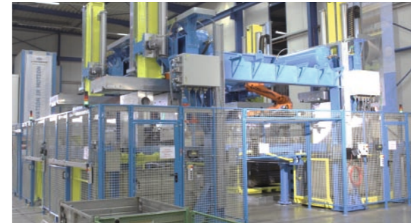
Automatic destacking of hot-formed pieces
