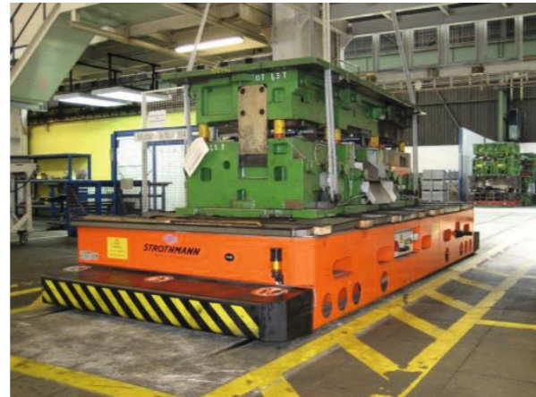
Transport carts with integrated drive for thermoforming tools
