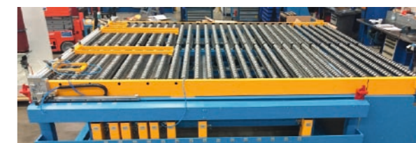
Centring station with servo-controlled centring fingers
