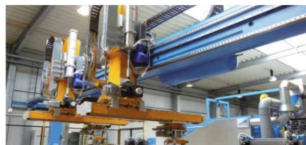
Blank destacking with double feeders and 4 blank carriages
