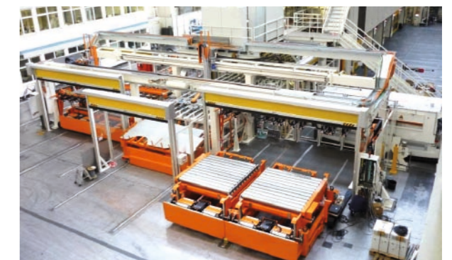
Blank loader with automatic pallet centring system
